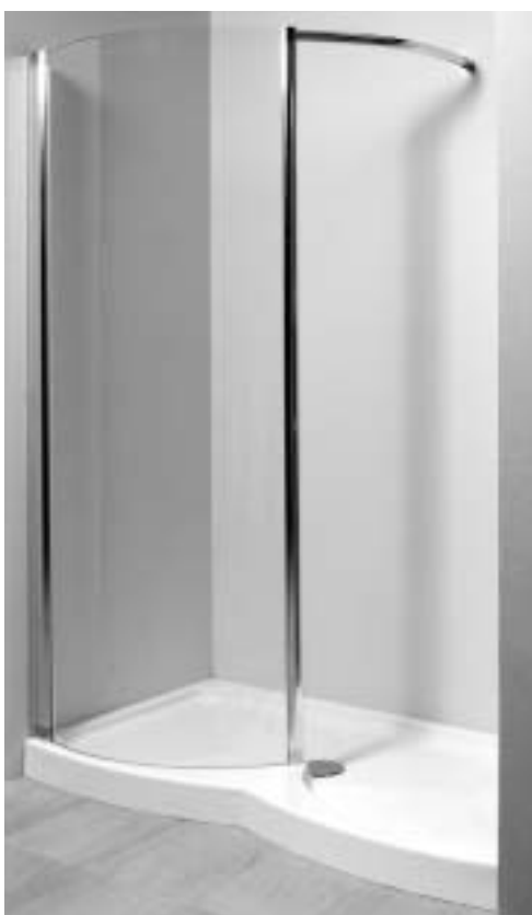
10 Alternative fitting in a recess without the end panel. Remove the ferrule connector cap with double spigot and replace with the single spigot version V8158. Swap to opposite ends of panel if required for left entry version.
