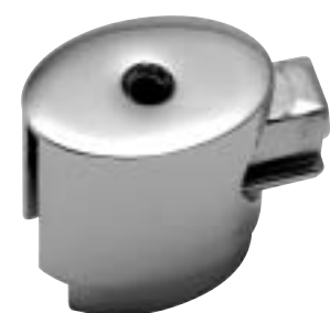
10 Alternative fitting in a recess without the end panel. Remove the ferrule connector cap with double spigot and replace with the single spigot version V8158. Swap to opposite ends of panel if required for left entry version.
