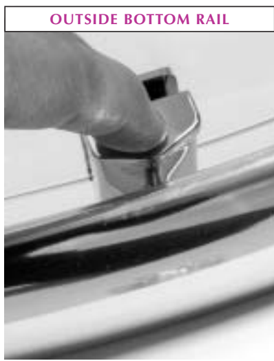
11 Working from the outside. Press down on quick release rollers & insert into bottom rail. Fit chrome covers V6103 to inside of single rollers. Press down on bottom rollers to gain easy access for cleaning
