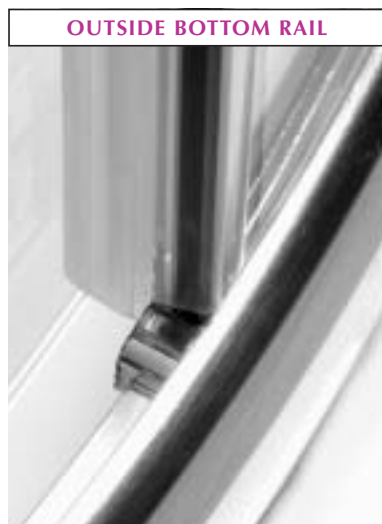
12 Fit upright short plastic seals on front of fixed panel V3104 & long seal on back of moving panel V3106. Ensure the bottom of the fixed panel seal V3104 sits tight to the fixed glass panel clip.
