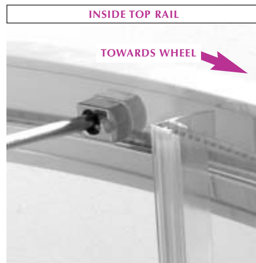
14 Fit SHORT roller stop V6104 into the pre drilled hole on the inside of the top profile. Insert cover caps V2111 to all roller stops.
