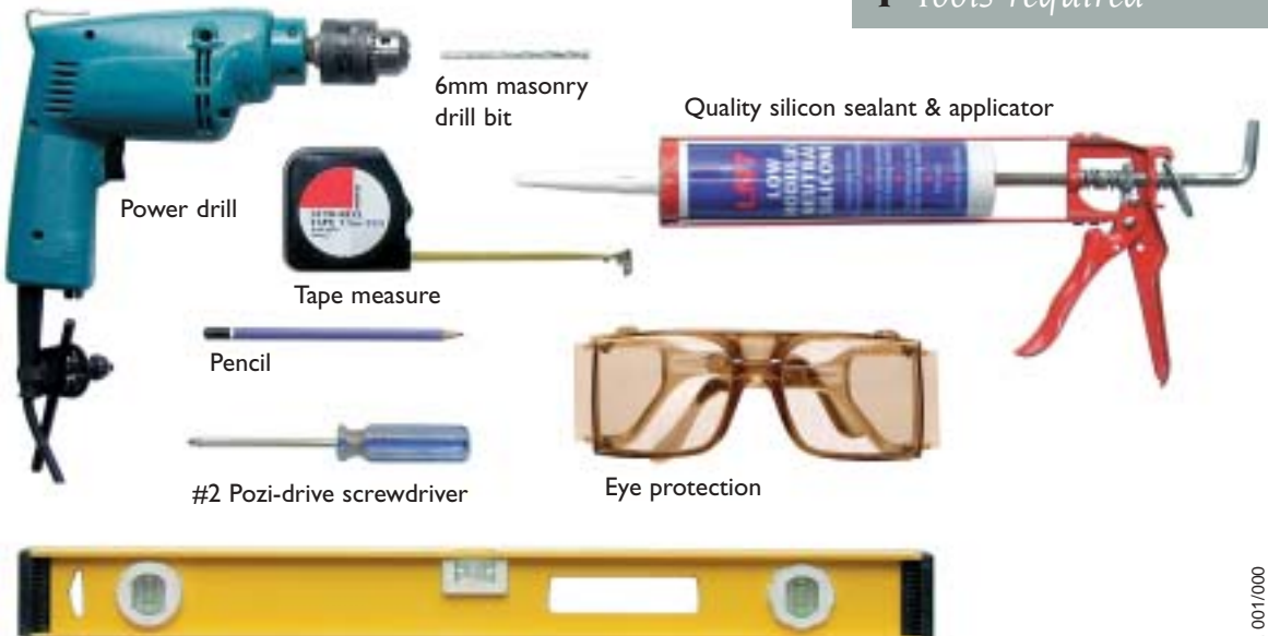
Spirit-level with horizontal & vertical level indicators
